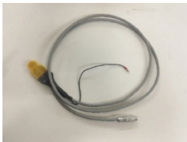
Fig. 6 Hot disc with bonding wire
